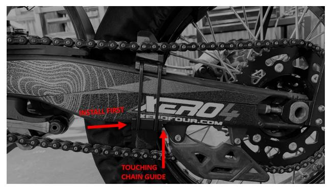
If any movement is noticed at this point in time, remove chain guide slowly and use supplied 3M VHB tape to shim as needed. OEM cast swing arms have variation from model to model.
